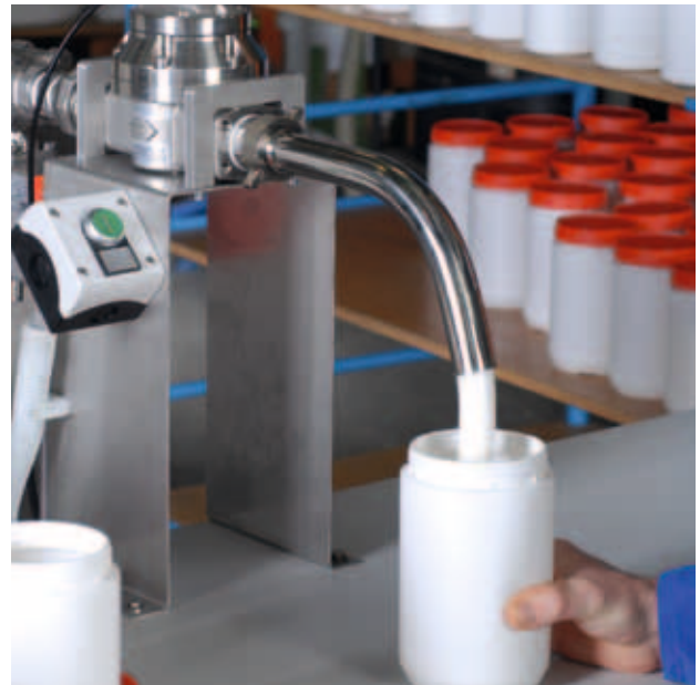
VISCOFLUX mobile – continuous transport (example: Vaseline).
